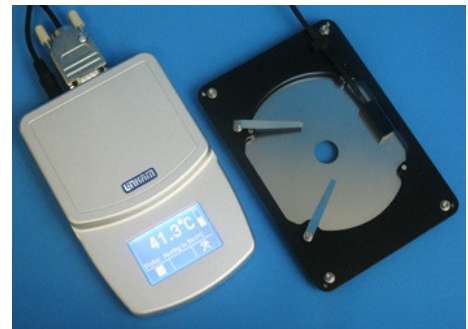
Fig 1 The DC95 and WSAX200 warm stage to fit Prior Optiscan
